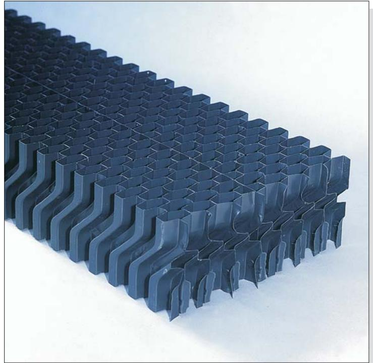
**THE H130 DRIFT ELIMINATOR**, with a geometry based upon 2 changes in the discharge airflow direction, is applied principally in situations of vertical airflow but can also be used for crossflow applications: it is constructed from preformed PVC sheets, subsequently made up into panels.
