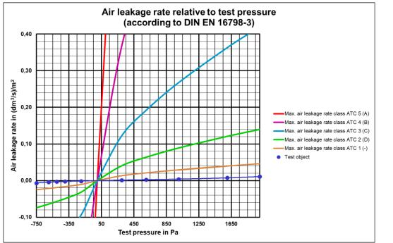
The air duct connection system "MEZ-SYPHON-FLANGE 30 - MEZ-BLUEMASTIC-GEL (138S)" achieves air tightness class D according to DIN EN 1507 and ATC1 according to DIN EN 16798-3.
