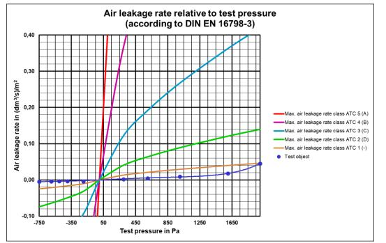
The air duct connection system "MEZ-SYPHON-FLANGE 20 - MEZ-BLUEMASTIC-GEL (128S)" achieves air tightness class D according to DIN EN 1507 and ATC1 according to DIN EN 16798-3.
